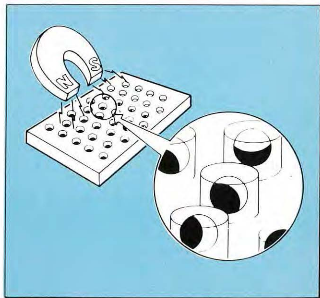
Fig 1 Principle of the magnetic particle display. Each spherical particle dark-colored in one hemisphere and light in the other is a tiny permanent magnet, free to rotate.
